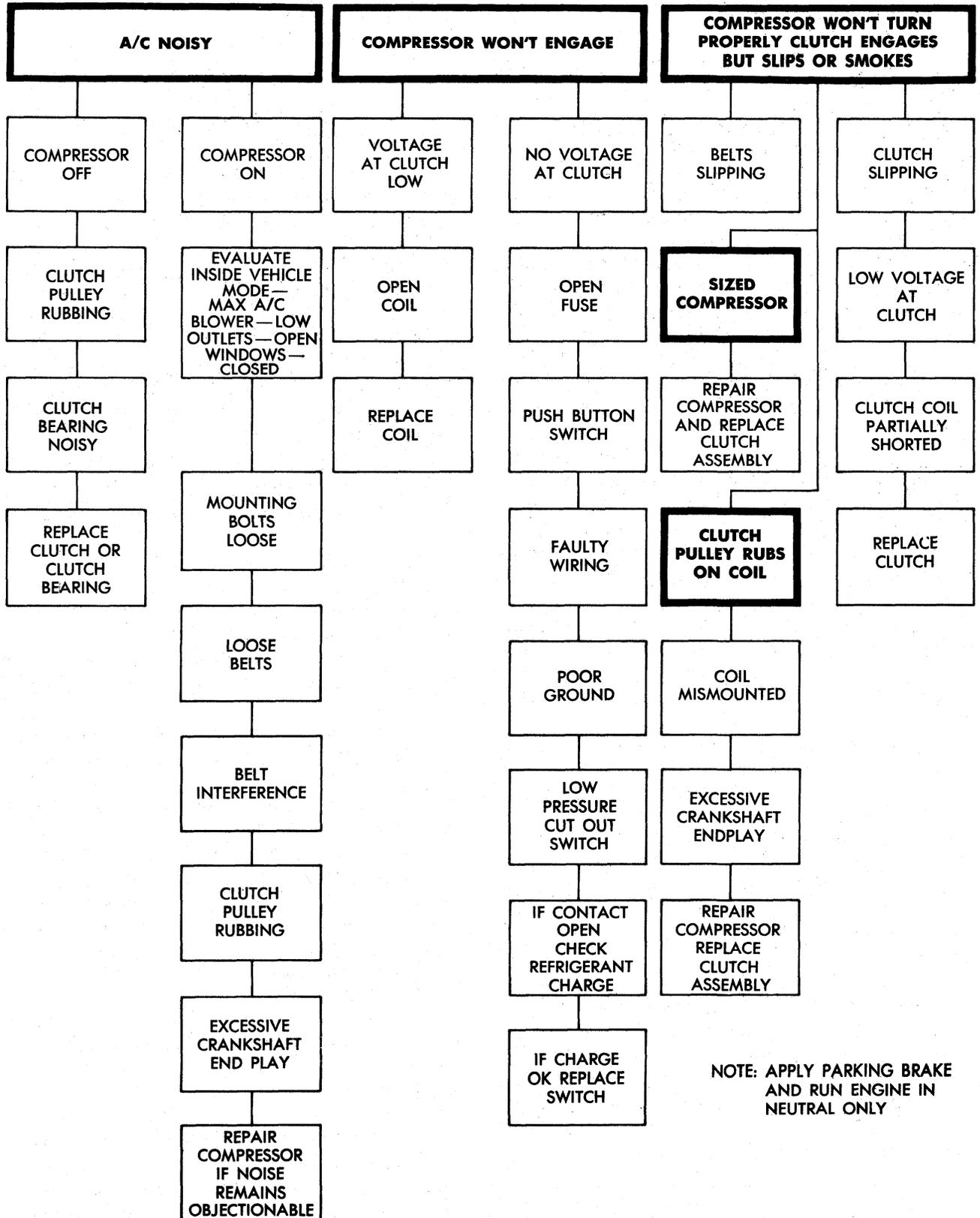
NOTE: APPLY PARKING BRAKE AND RUN ENGINE IN NEUTRAL ONLY
