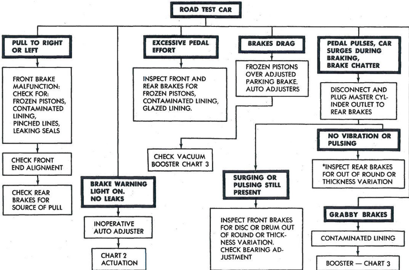
\*PULSATION CAUSED BY REAR BRAKES MAY BE ELIMINATED OR REDUCED BY ROTATION DRUM (REAR) TWO STUDS ON AXLE FLANGE.
