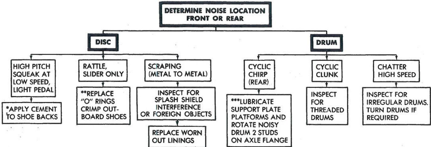
\*APPLY MOPAR CEMENT PART NUMBER 3683897, OR EQUIVALENT, TO SHOE BACKS AND TO PISTON AND CALIPER FINGER CONTACT AREAS. REMOVE ALUMINUM GASKET IF SHOE IS SO EQUIPPED.
