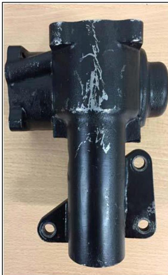
There are other options available and LVVTA has seen an increase in aftermarket steering component manufacturers having their own steering box housings manufactured using a casting process (the same as OEM manufacturers), thus completely eliminating the need for any welding.
