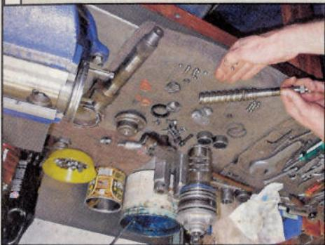
(Left) Here's a box's myriad com-ponents blueprinted and ready for assembly at Firm Feel, Inc., with worn parts replaced, and Firm Feel's firm free Stage II reaction springs (arrow). Assembly skill and parts selection is what separates the men from sloppies—tighter, more repeatable ball joints—26 of 'em, to be exact, to build a fresh, stiffer steering. (Right) It takes lots of balls—grade E52100 alloy steel balls, quality high-carbon aircraft (chromium) box, FF uses only 100% new, bearings—
