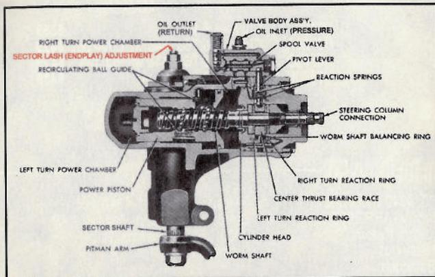
This factory cutaway clearly shows the position of the sector lash adjustment (and locknut), just forward of the valve body's return nipple. But how, exactly, do you adjust the lash, to eliminate wheel freeplay? Yeah, how?
