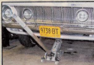
Place the wheels in the dead-ahead position, engine off, wheels off the ground. Now start the engine while observing the steering wheel. There should be zero movement of the wheel as the engine starts. If there is the slightest movement, the valve body needs to be adjusted.
