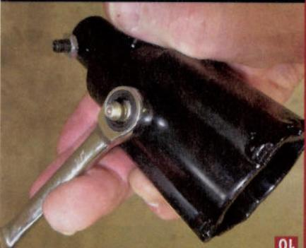
One trick we've used for decades: Add a grease fitting to the coupler. Drill a 1/32" hole at the bottom of the inner machined area.
