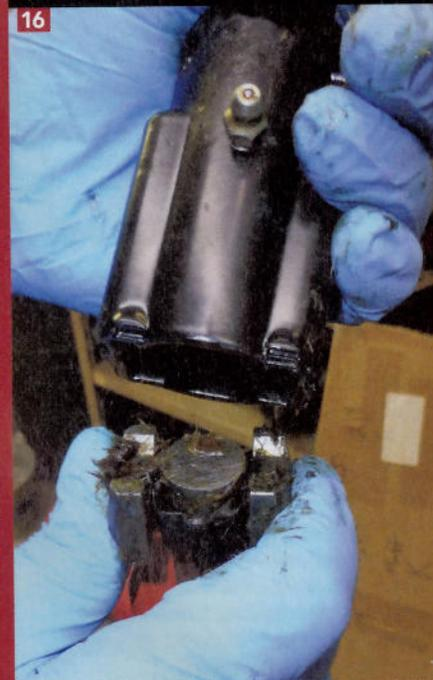
**16** Assemble the pot coupler to the shaft using the new components provided. Slime with long fiber grease, this is less critical if you have wisely installed a grease fitting.
