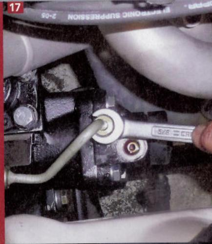
**17** Hook up both hoses. The one shown is the pressure side. Our original hose screwed right on using Bergman's adapter fittings.
