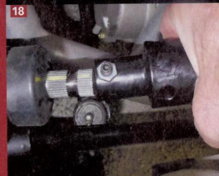
**18** Loosely reinstall the column back into the car. Slip the coupler onto the box's splines, insuring the 12 o'clock on the wheel is aligned with your high spot mark. *This is important!*
