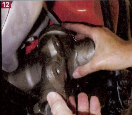
**12** Drain the lube, then take out the mounting bolts (3), duh. Depending on model, engine, headers, etc. you may need to remove the left header or manifold, or jack the engine up a bit. It may be easier, in some instances, to remove it from the top.
