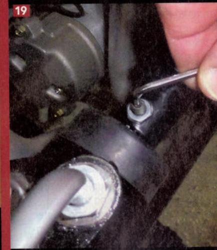
**19** Tighten the setscrew securely, then the jam nut.
