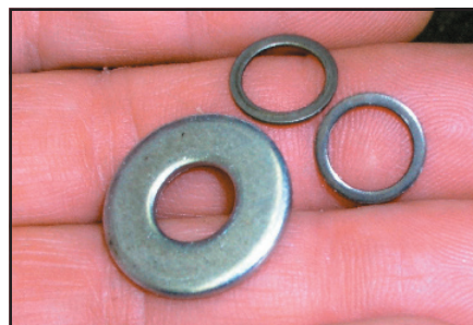
(14) The shims are ⅜" ID, ½" OD (exactly, nothing metric here!) A hardware store ⅜" flatwasher (left) has way too large of an OD. You'll need to either grind down the OD (need not be precise), or start with a ½" OD washer and drill the center hole to ⅜". If you're shooting in the dark (no pressure gauge), we'd start by adding about 0.062" to whatever you find in your valve. Brass might be easier to work with than steel and would be fine.
