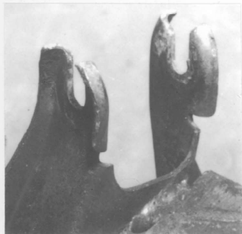
Left-hand, or driver's side, engine mounting perch
