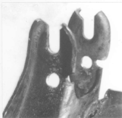
Left-hand, or driver's side, engine mounting perch
