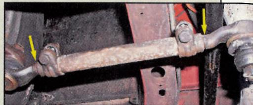
At this point, the wheels should be straight ahead and the amount of visible thread approximately equal on *all four* tie rod ends. If not, your front end alignment guy did a "workaround" because something's not right. Possible problems are an incorrectly assembled pot coupling (inverted, more on that next issue), the aforementioned steering wheel installation snafu, frame, chassis, or linkage damage, or, more common than you might think...
