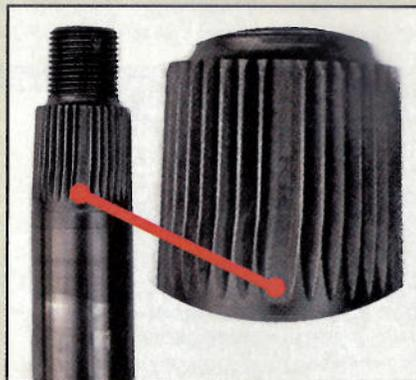
...a twisted chuck (steering box) sector shaft. Nasty!
