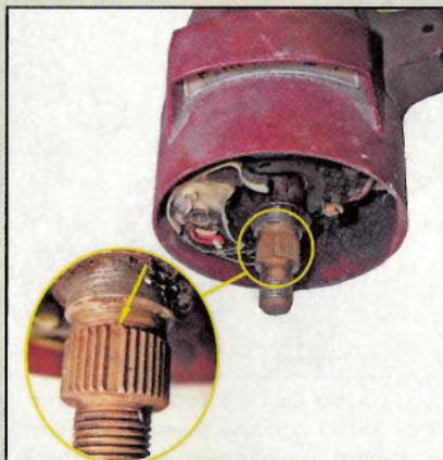
At this point, the steering wheel's master spline *must* be at 12 o'clock. If there's any doubt about this (maybe some idiot filed a new, incorrect master spline, or an after-market wheel adapter, which frequently have no master spline index, was installed incorrectly), remove the wheel nut and have a look (you can see the column shaft master spline without pulling the wheel as long as you remove the nut).
