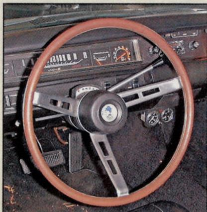
To check that all components of the steering system are lined up correctly, begin with the steering wheel pointing straight ahead.
