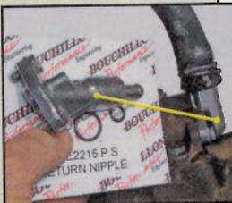
Ditto the pressure fitting. In most cases, we'd advise spec'ing a pressure hose for your engine and a Sag pump, in a circa-early-'70s car they are readily available. If the pump end doesn't mate to your chuck's fitting, Bouchillon has your back.
