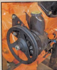
it's out there. Bouchillon seems to be the one-stop shop. They even carry the hard-to-find thin-pattern pulley-mounting locknut and special pulleys to adapt the later 3/4" "smooth" (press-on pulley) shaft pump to early Mopars. Hoffman's Winners Circle makes a super nice bracket kit that also includes 100-point resto-correct mounting hardware (bolts, etc.) and 440 Source has low-cost brackets.
